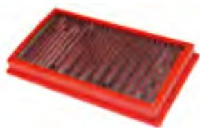
Let the filter totally absorb the oil. This can be checked by checking the evenness of the red color on both sides of the filter.
