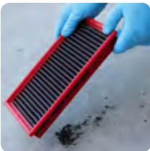
Remove the filter and tap it gently on a solid surface to remove the largest impurities (such as grass, gravel and bugs) and clean the airbox. Be careful to avoid damaging the filtering element.
