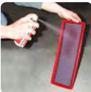
Spray the oil evenly onto both sides of the filtering element from a distance of 15 cm.
