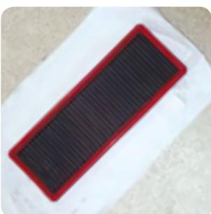
Let the filter dry naturally outdoors without exposing it to direct sunlight. The filter is dry when it no longer releases water or humidity. This can be checked using compressed air, gently and from a safe distance in order to avoid damaging the cotton fabric.
